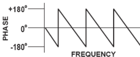
Figure A-15. Linear Phase with Frequency Waveform
