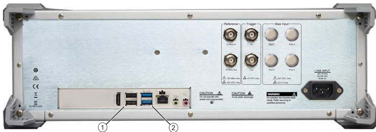
Figure 2-3. Rear Panel Keyboard and Mouse Connections
